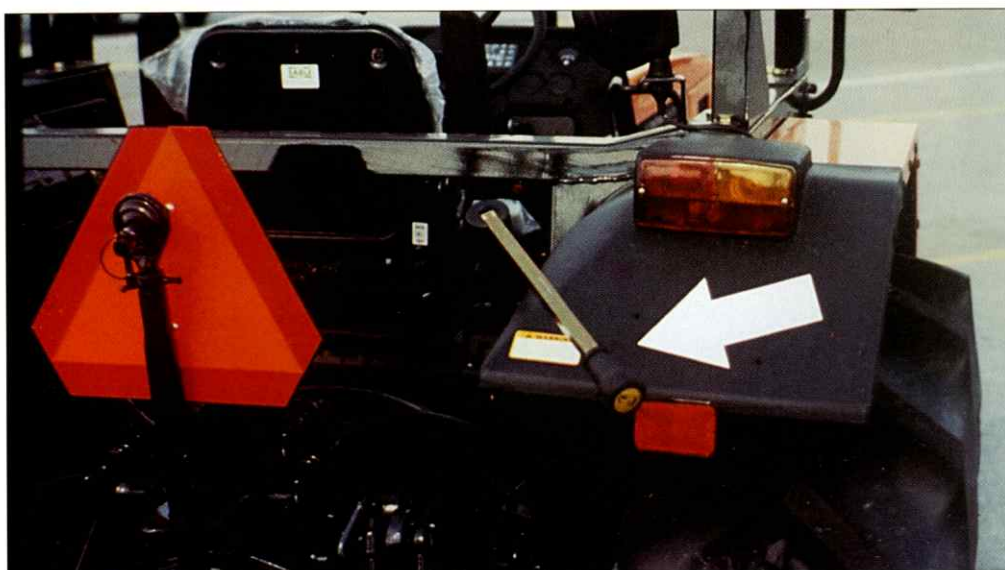
REMOTE 3-POINT CONTROL
