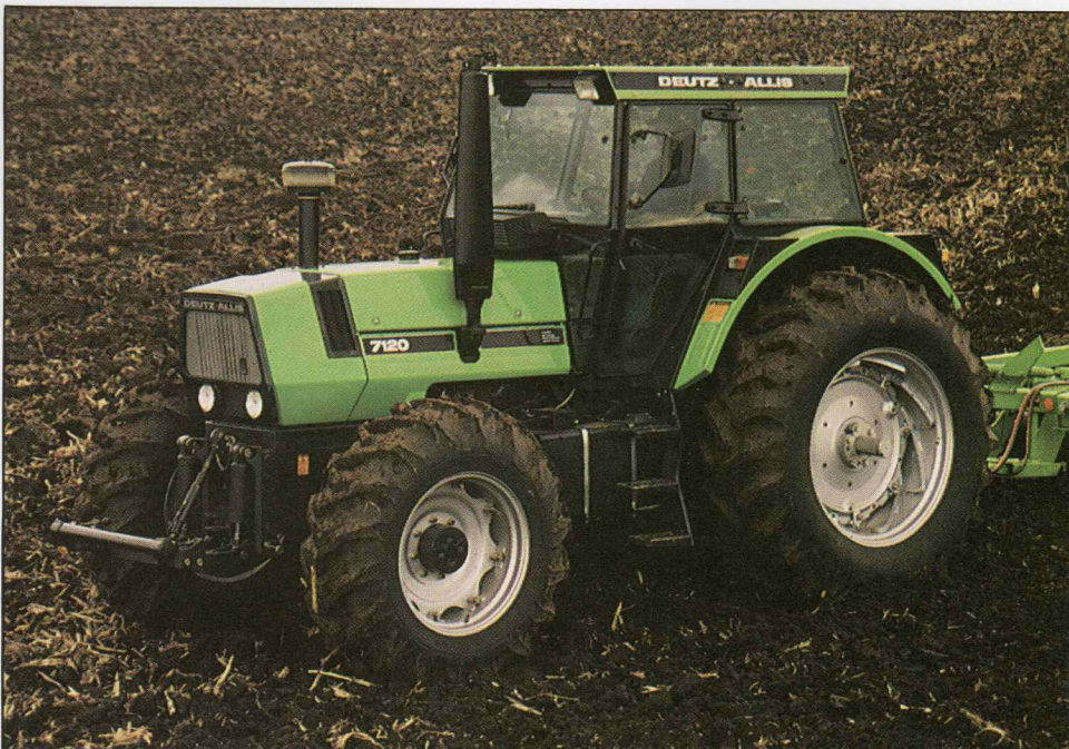
Top: All-Wheel Drive improves fuel efficiency and traction; bar-type axle provides variety of tread widths.
