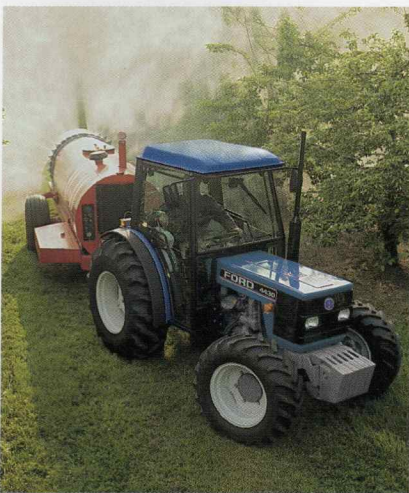
Dimensions of Model 4430 with cab: Height, 85.6 inches. Width at fenders, 44 inches. Width at top of cab, 37.5 inches.
