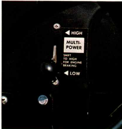
12-speed Multi-Power transmission offers shift-on-the-go convenience and wide choice of speeds. Available on any MF 1085 or MF 285.
