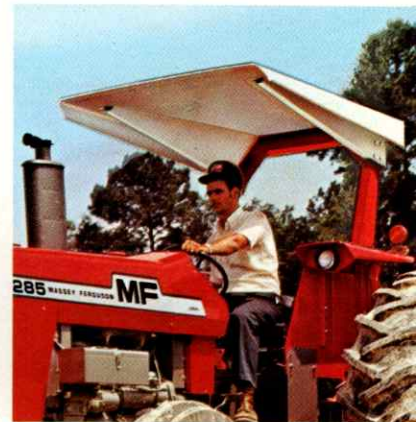
ROPS and canopy available for shade and protection against accidental roll-over.
