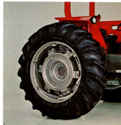
Power adjust variable tread (PAVT) wheels with some tire sizes on MF 1085 and MF 285 put engine power to work changing tread spacing. A wide variety of front and rear tire sizes are available.
