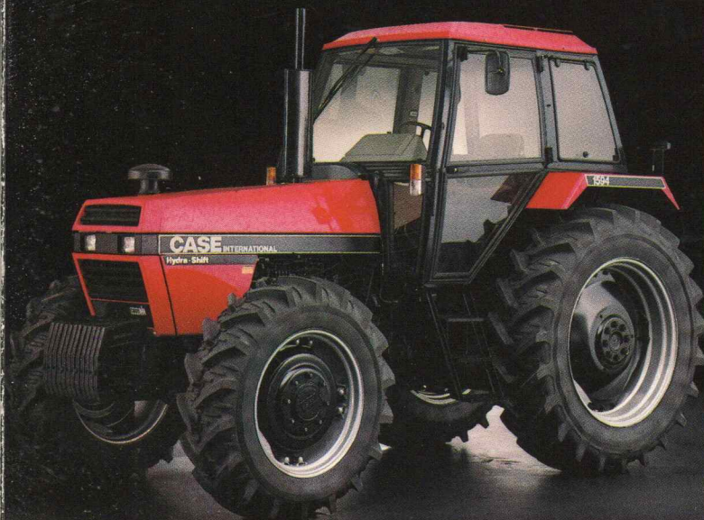
1455XL 4WD 145 DIN hp turbo-charged engine, XL control centre and turbo clutch transmission.
