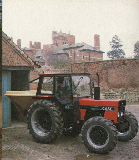
585L 4WD 59 DIN hp with low profile economy cab, synchromesh transmission.
