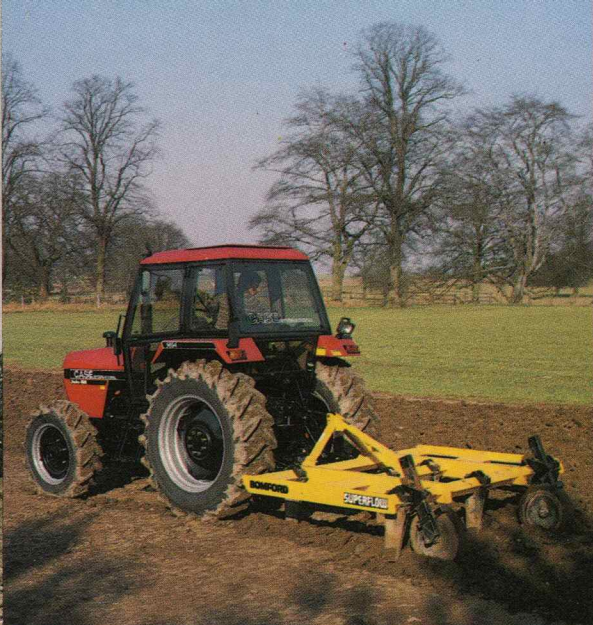
1494 4WD 83 DIN hp turbo-charged engine, hydramatic transmission and split cab facility.
