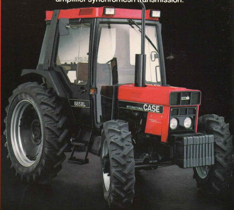
885XL 4WD 82 DIN hp with XL control centre, and torque amplifier synchromesh transmission.
