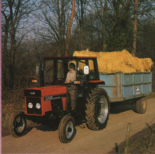
485L 52 DIN hp with low profile economy cab, synchromesh transmission.
