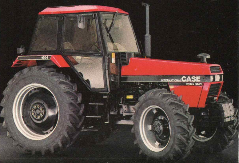
1694 4WD 108 DIN hp turbo-charged engine, hydrashift transmission and lowerlink sensing.
