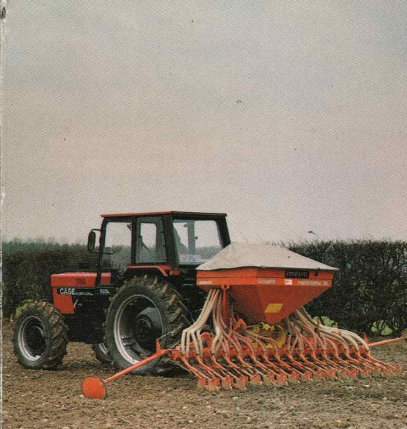
685L 4WD 69 DIN hp with low profile economy cab, synchromesh transmission.
