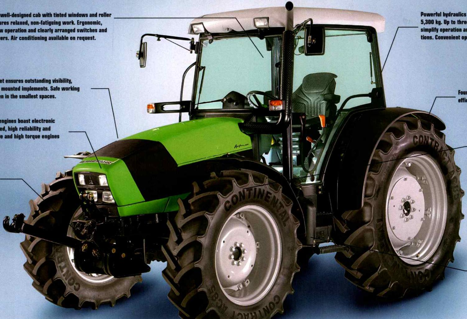
Powerful hydraulics with lifting forces of up to 5,300 kg. Up to three additional remote valves simplify operation and widen the range of applications. Convenient operation using single levers.
