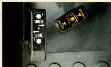
The PTO speed is pre-selected from the cab on the left of the driver's seat.
