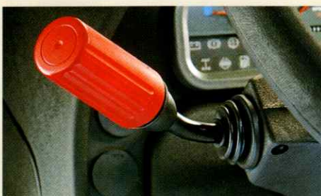
Changing of the driving direction forward or reverse without clutch.
