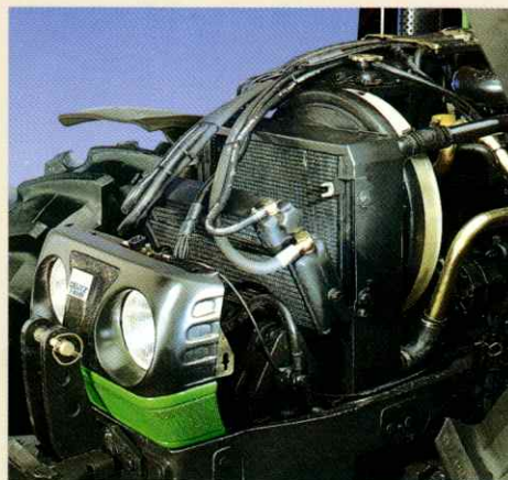
The easy to maintain cooling unit is accommodated in an area separate from the engine.
