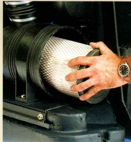
The new position of the air filter permits the direct access without tool.
