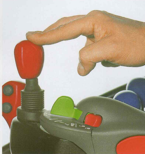
Powershift: Convenient press-button shifting with the optional shifting lever integrated into the armrest.
