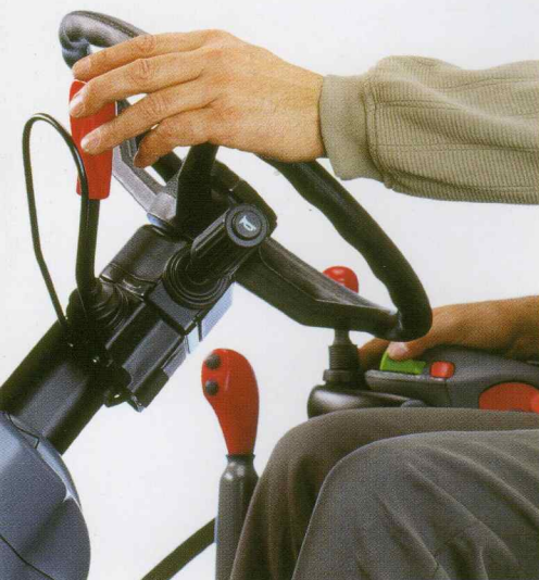
PowerShuttle: Forward/reverse travel without actuating the clutch. A significant advantage for many daily jobs.
