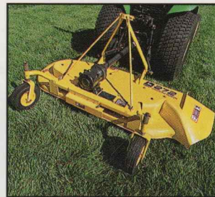
272 and 261 Rear-Mount Mowers Three-point-hitch grooming mowers come in 5- and 6-foot widths and are built of reinforced stamped steel. A 60-inch mid-mount mower is also available.
