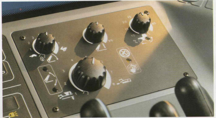
The rugged ElectroLink draft control panel is clear and concise. From top left: lowering speed and Dynamic ride control, maximum lift height, wheel slip override, and draft and position control intermix.
