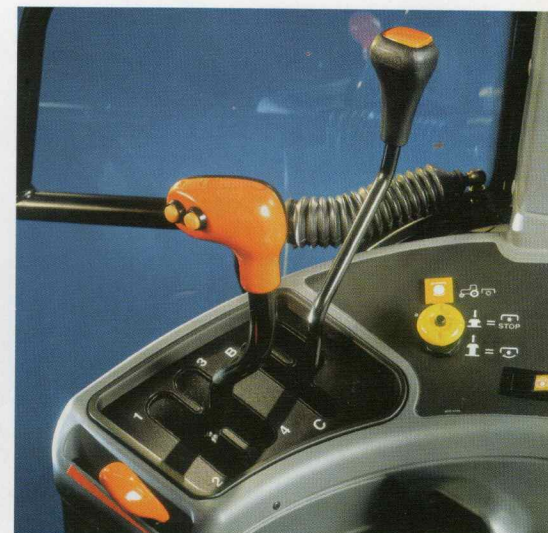
Dual Command offers flexible speed control with two powershift speeds in each gear. The power shuttle control is on the left of the steering column.
