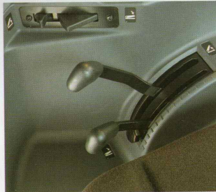
Flexion bar draft control with Lift-o-matic for easier turning at the end of the field.
