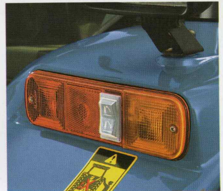
External control switches aid attachment of implements.
