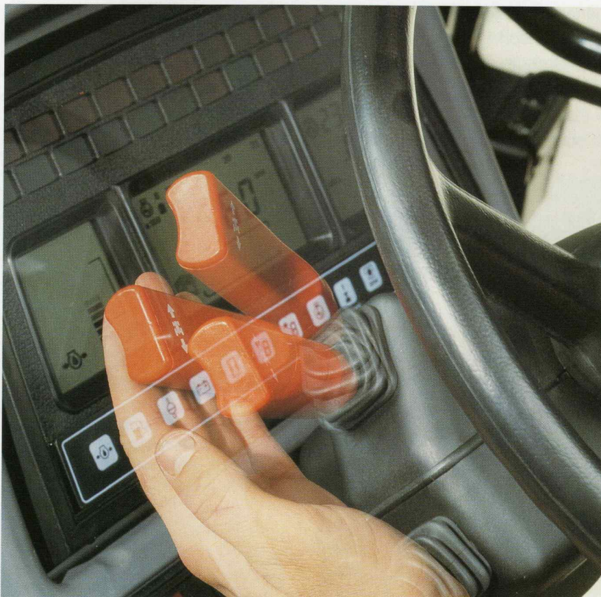
Dual Command offers flexible speed control with two powershift speeds in each gear. The power shuttle control is on the left of the steering column.
