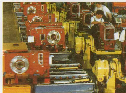
The transmission and rear axle of the Series 60 are transported between assembly positions by automatic carriages.
