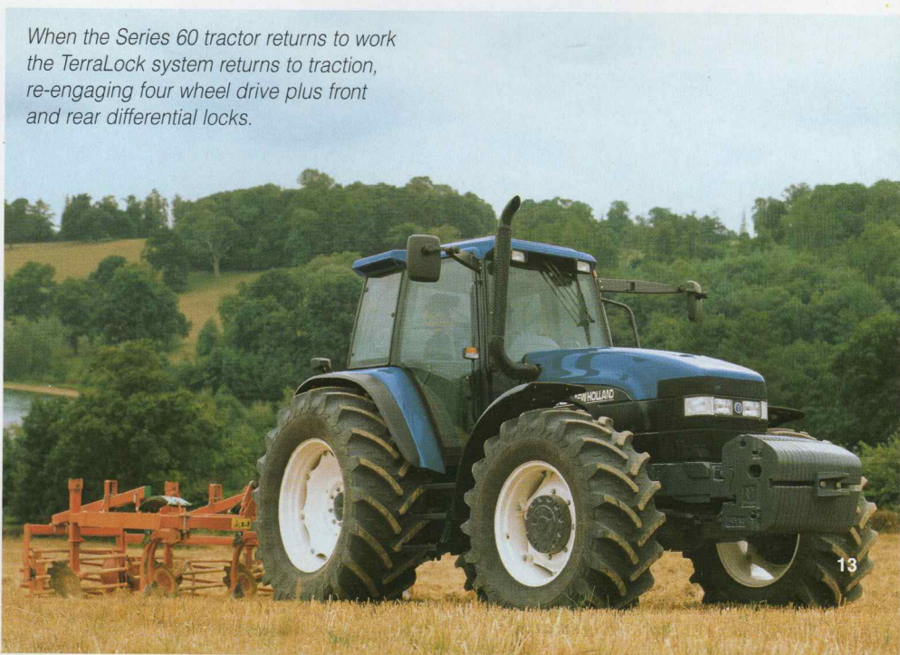
The advanced TerraLock system can automatically shift between traction and manoeuvrability. It also provides permanent engagement of four wheel drive and front and rear differentials
