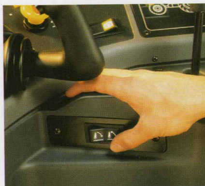
The Lift-o-matic system raises and lowers the implement to make turning at the end of the field easier.
