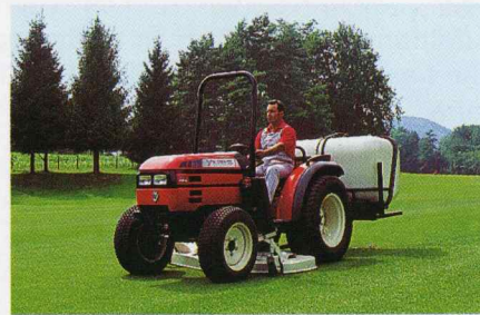
3-BLADE MOWER . (working width 1500 mm). Cutting height 12 to 90 mm.
