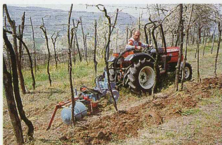
ONE-FURROW PLOUGH , mechanical or hydraulic. Working depth 300 mm.
