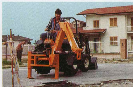
BACKHOE . Working height 2300 mm. Working depth 1800 mm.
