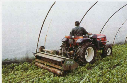
SHREDDER . Working width 1500 mm.
