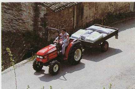
TRAILER with 3-way hydraulic tilt. Farm version 2500 x 1000 mm. Garden version 2300 x 1200 mm.
