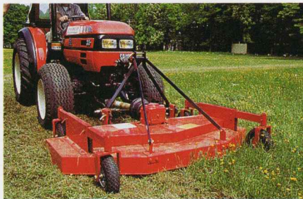
3-BLADE MOWER . Working width 1800 mm.
