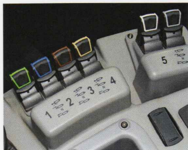
Electro-hydraulics in optional six valve configuration.
