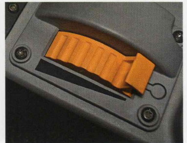
A simple responsive hand throttle helps you set your RPM.
