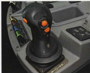
Four function powershift lever for quick control
