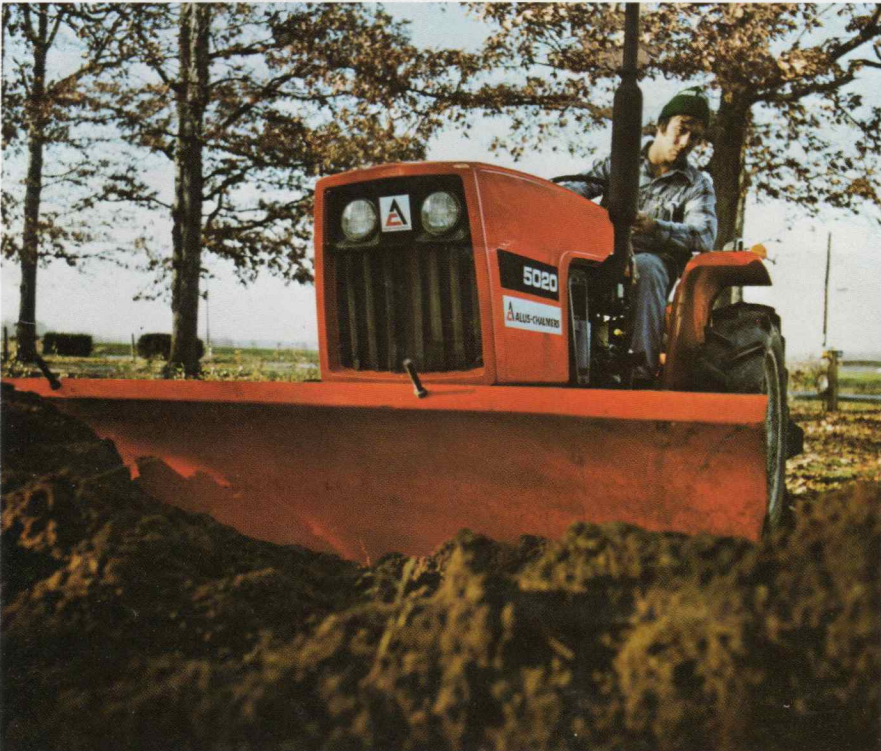
Powerful 5020/5030 tractors handle even tough dozing jobs. Front blade is heavy steel, angles right or left 0° to 30°, and clears a 72" width straight ahead. Maximum digging depth is 2". Replaceable cutting edge.
