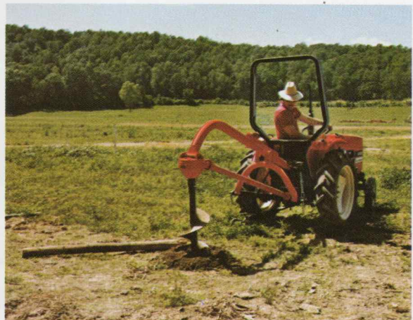
Four-foot-long post hole digger available with auger sizes of 6", 9" and 12". Pilot tip is hardened alloy steel. Makes easy work of tough fencing or shrub-planting jobs.
