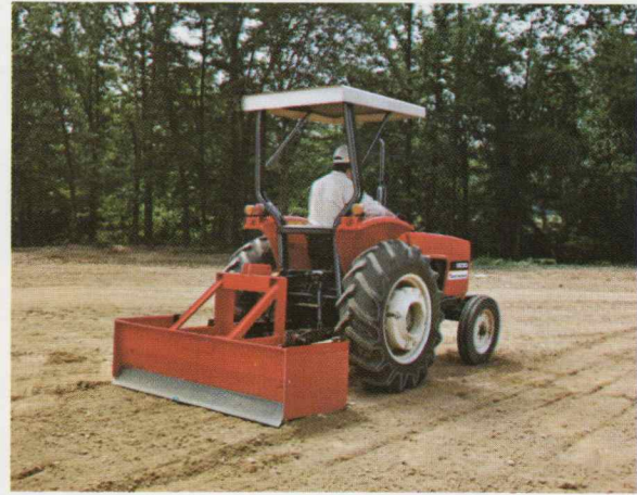
Box Scraper makes short work of leveling, grading, backfilling and scarifying. 66" wide. End width is 24", end depth 18½". Cutting edge is ½"×6"×66". Replaceable scarifying teeth are standard.
