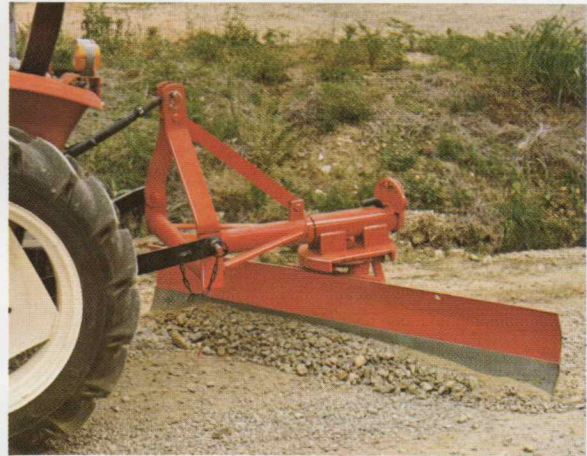
Scraper and grader blades come in 72" cutting widths... blade height is 13½" with a cutting edge of ½"×6"×72". Blade can be angled 60°, 75° or 90° to direction of travel; heavy-duty blade angles 45°, 60°, 75° or 90° and has tilt adjustment. Reversible cutting edgers on both blades.
