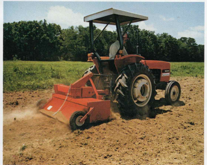
Build a fine seedbed in a hurry—with a rotary tiller. Unit is hydraulically raised or lowered, easy to lift over rocks.
