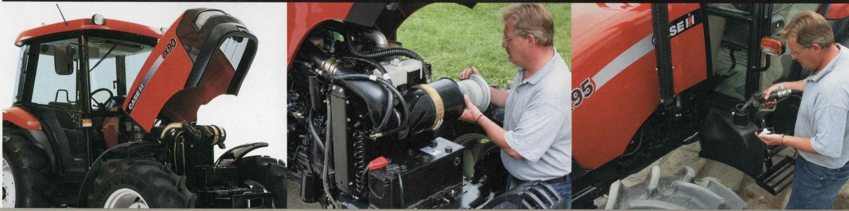
The air filter is readily accessible and quick to service.
