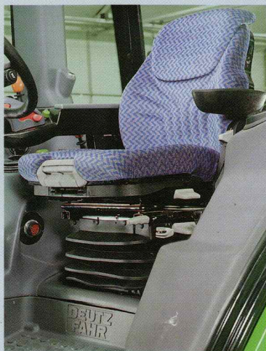
Front axle and cab suspension and Grammer-Maximo seat
