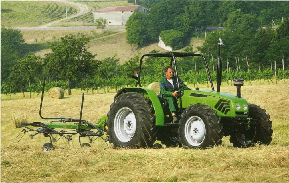
has modulated hydraulic servo-control for precise and effortless drive take-up. The synchro, ground speed PTO with its independent output shaft can be used simultaneously, uniquely ensuring drive to both machine mechanism and ground wheels.
