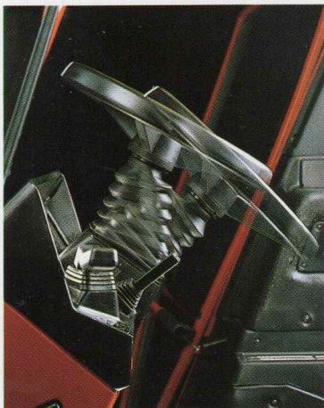
Steering wheel with adjustable height and rake according to height and preferred driving position.
