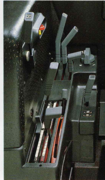
Console on the operator's right with the controls/adjustments of the hydraulic lift and auxiliary control valves.
