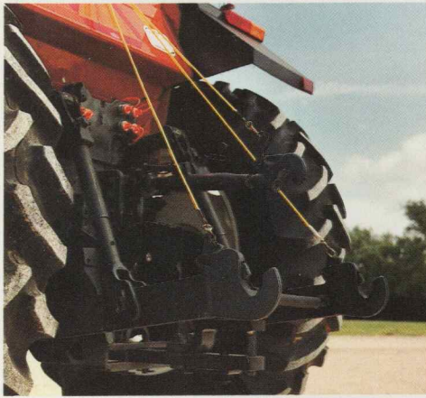
Walterscheid quick attach hitch (standard on 160-90 and 180-90) permits faster, easier attachment of mounted implements.
