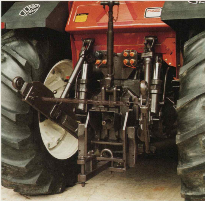
Walterscheid quick attach hitch (standard on 160-90 and 180-90) permits faster, easier attachment of mounted implements.
