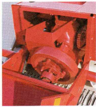
Slip clutches on transmission and pickup assembly protect all major components.
