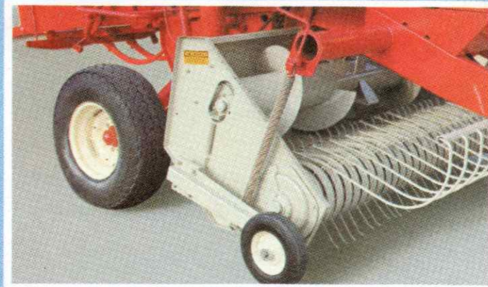
Standard gauge wheels and flotation springs, on both ends of pickup, give ground-hugging action and clean sweep of windrows.
