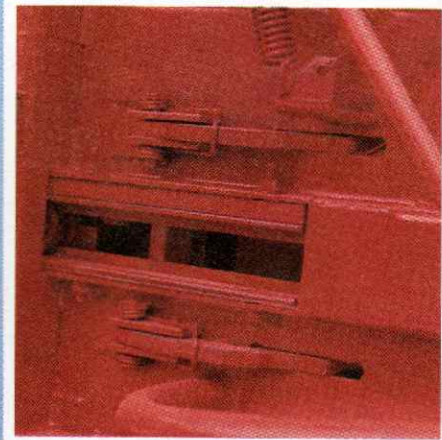
Hay dogs feature rubber silencers to cut down "clacking" noise common to most conventional balers.
