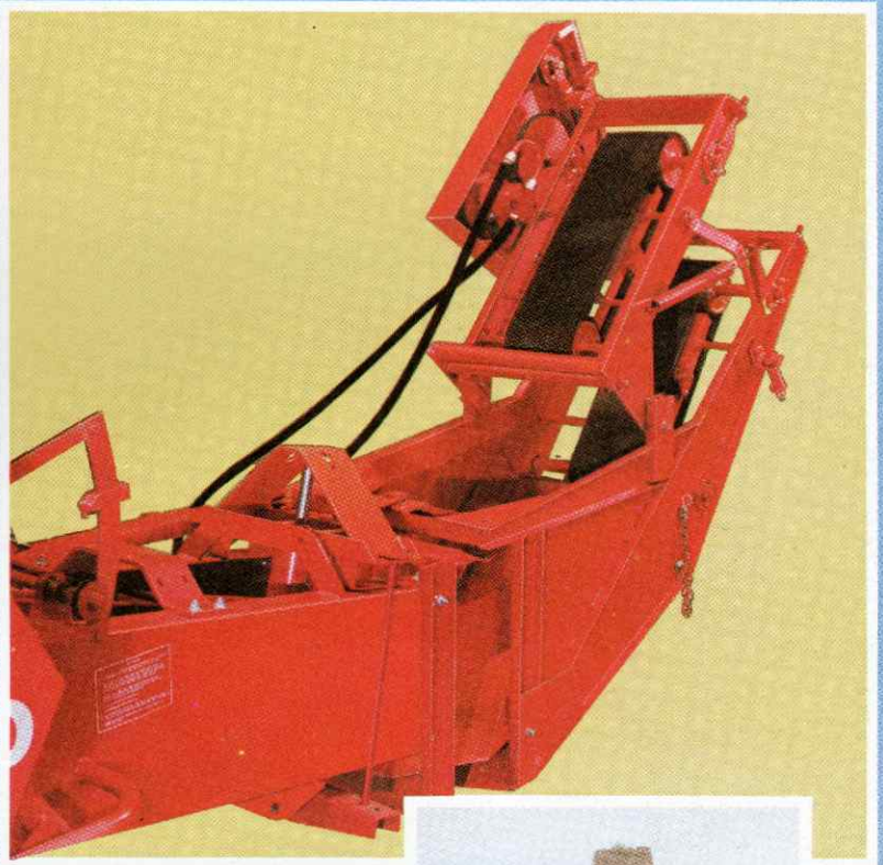
Single chain drive system powers pickup, Packing Fingers and Stuffing Fingers. Stuffing Fingers are cycled with each plunger stroke. Chain is driven direct from the heavy-duty transmission. Positive roller chain drive keeps all bale-forming mechanisms in time. Plus, drives are all on same side of baler for fast, easy servicing.
