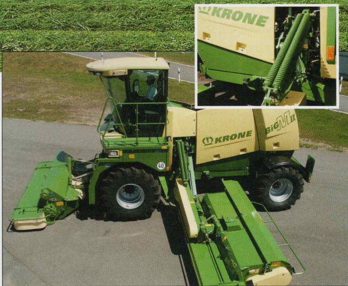
Optimum guidance: Spring relief packages reduce the contact pressure of the side mowers and provide the optimum contour following on the ground and are adjusted manually by means of a bolted central coupling bar. Hydraulic adjustment is available as an option.
