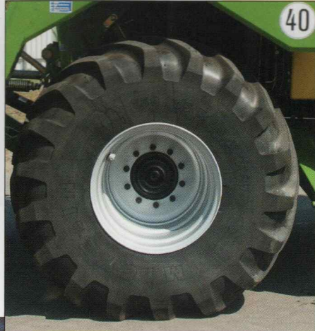
Easy on the turf: The large-volume tyres – 750/65 R 26 at the front, 600/65 R 26 at the back – ensure optimum protection of the precious sward. The large contact surface of the BiG M II tyres leaves no tracks or ground compaction.
