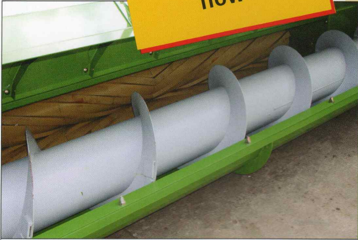
The insides: The crop is transferred from the mower via the CV or CRI conditioner into the conveyor augers and then transferred on to the middle swath.
