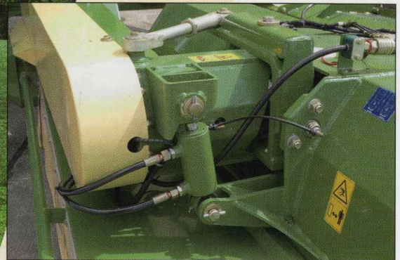
FlexiCut: Hydraulically set cutting height option. When working in varying conditions, a previously saved cutting height can be recalled at any time to ensure neater working.
