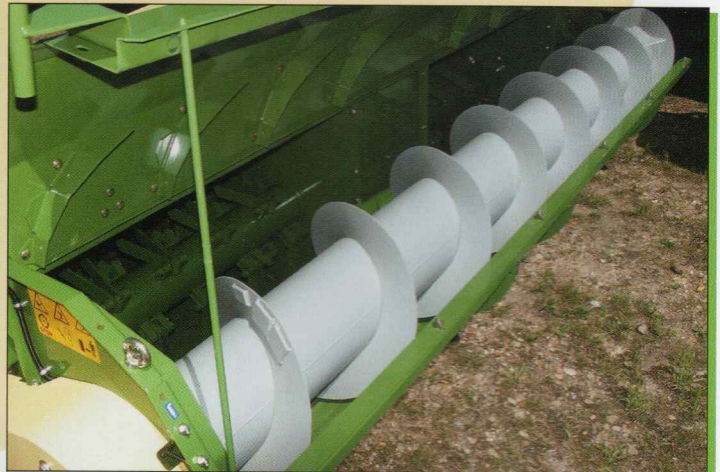
View of the guide plates: Guide plates are integrated in the hood for reliable conveyance of the crop to the centre.
