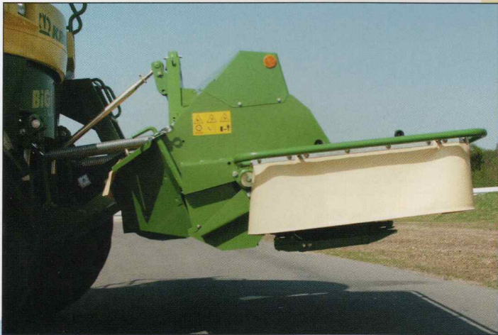
Pushing ahead of the rest: The integrated "A" frame with high upward and downward clearance, together with adjustable tension springs and long skids ensures optimum ground adaptation in the toughest conditions. The result: A clean cut.
