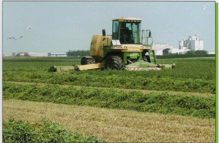
Clean: The BiG Swath System with a CRi conditioner in lucerne. Without touching the ground, the augers transfer the crop on to the swath produced by the front mower.
