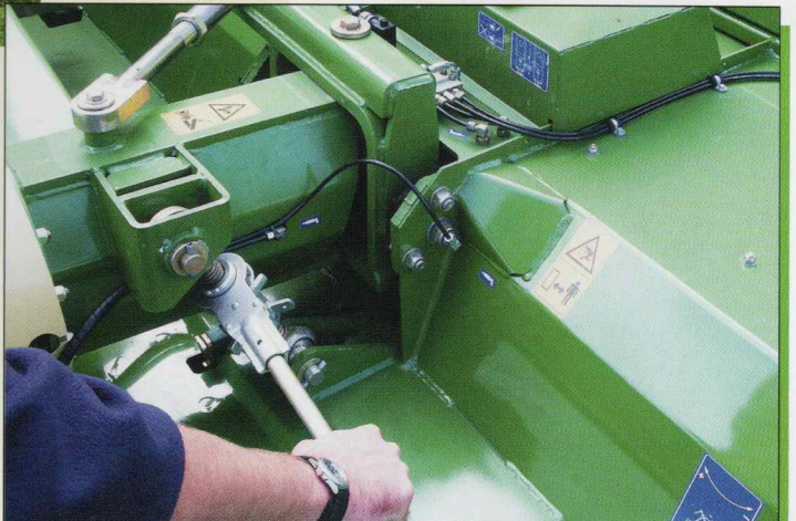
One movement of the hand: Adjustment of the cutting height on the side mowers is fast and easy. This allows you to quickly adapt the mowers to the local conditions.
