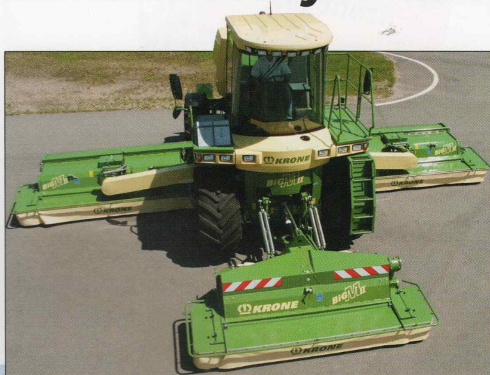
BiG M II, the mowing giant: 9.70 m mowing width with three EasyCut mower units and CV high-performance conditioners or 9.00 m with CRI conditioner rollers. The mower units all function independently with a clean cut always guaranteed.
