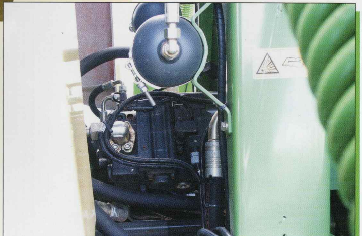
Infinitely variable drive concept: Two pumps for the all-wheel drive. The front and rear axles are driven separately enabling the BiG M II to handle even the roughest terrain.
