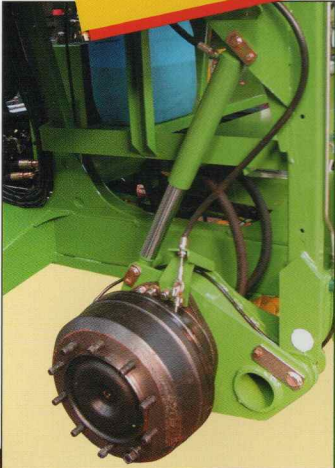
Spring-mounted front axle: The BiG M II has a hydro-pneumatic spring-suspended front axle as standard equipment. It provides not only for a quiet, comfortable driving behaviour, but also for increased ground clearance when mowing.
