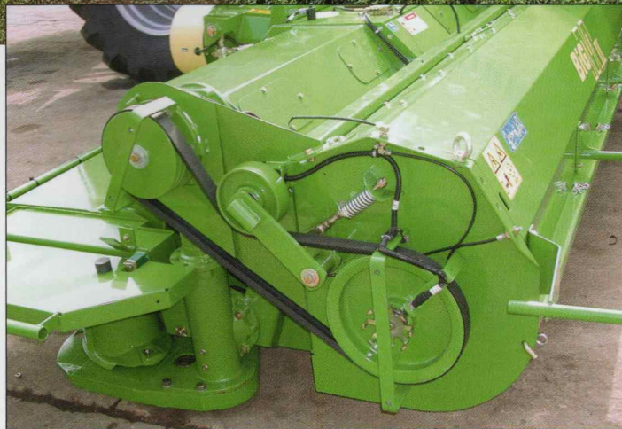
View of the drives: The BiG Swath System uses a powerful and reliable belt drive system. For wide swath deposition, the BiG Swath System can easily be removed and replaced by a conditioner cowling.
