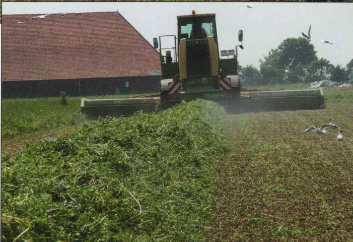
Closed: The view from the rear shows the compact unit, completely enclosed, that reliably channels the forage to a swath with a width of 1.80 m.
