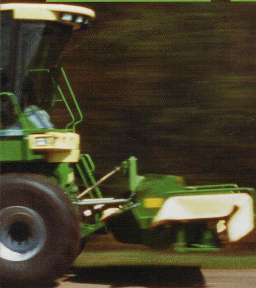
Spring-mounted front axle: The BiG M II has a hydro-pneumatic spring-suspended front axle as standard equipment. It provides not only for a quiet, comfortable driving behaviour, but also for increased ground clearance when mowing.
