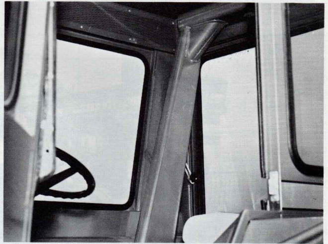
Slide 60 — Inside View of Cab Showing Safety Frame
