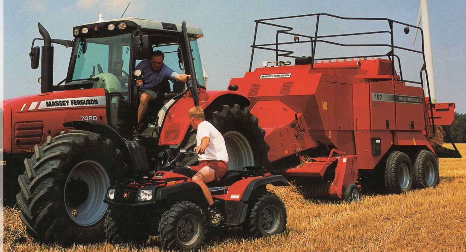
MF185 Series II produces bales of 0.88 m x 0.80 m section up to 2.50 m long and will bale silage, hay, lucerne and straw.
