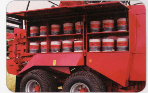
There is plenty of room for twine storage on each side of the baler.
