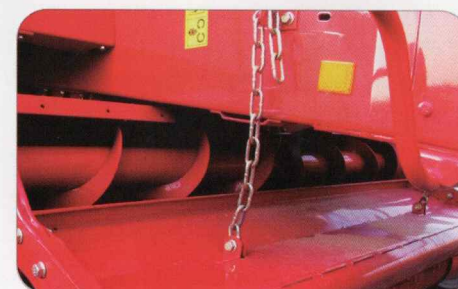
MF 185 SII and MF187 balers with cutter option have a solid high performance windguard for smooth crop flow.
