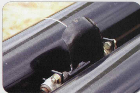
The bale drop indicator shows when the bale has dropped off the end of the roller bale chute.
