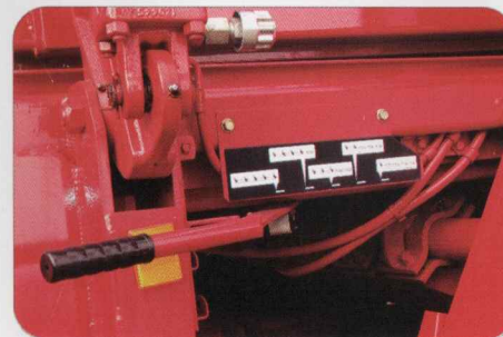
On the MF 185 SII and MF 187 the bale ejector lets you remove the last bale or clear the whole chamber. Just select the required number of teeth with this lever.
