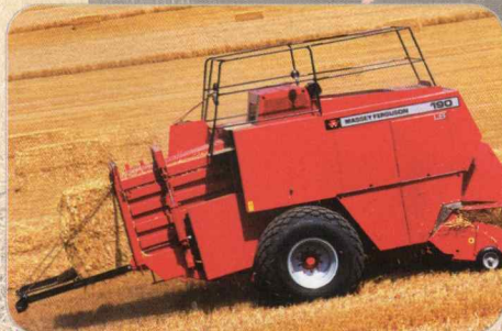
The MF190 produces bales 1.27 m x 1.20 m section up to 2.74 m long and will bale hay and straw.
