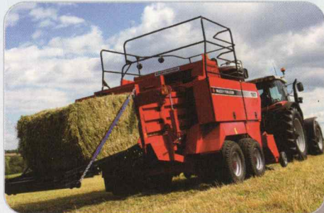
The MF187 produces bales of 0.88 m x 1.20 m section up to 2.50 m long and will bale silage, hay and straw.
