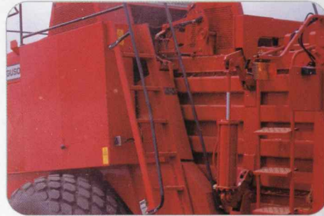
Automatic density control measures the load on the plunger and uses the hydraulic rams on the bale chamber to maintain an even density throughout the bale.
