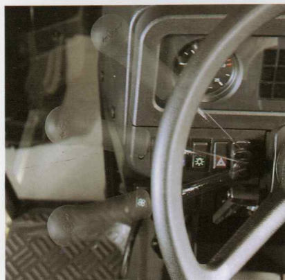
Above: The shuttle lever is conveniently placed to the left of the steering column, leaving the right hand free for gear changing and spool valve operation
