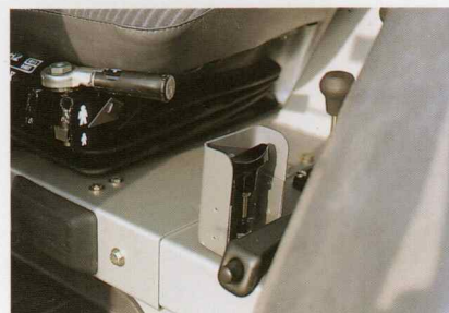
Below: Handy creeper gear selection is by a simple mechanical lever
