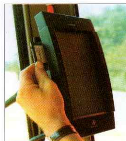
Fig. 1. The Data Card is used to transfer information from the combine to the farm computer
