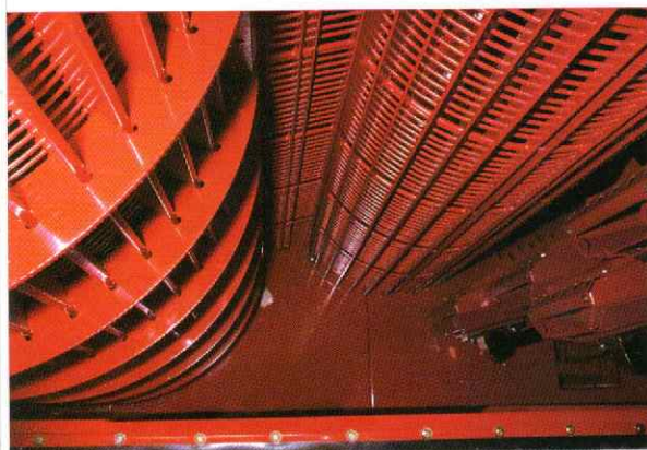
RS models benefit from the additional separation area of an extra grate and concave
