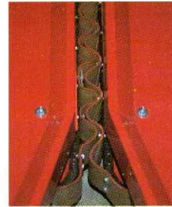
MF Sunflower table with (inset) detail of the gathering belts. (Some versions are fitted with gathering chains)
