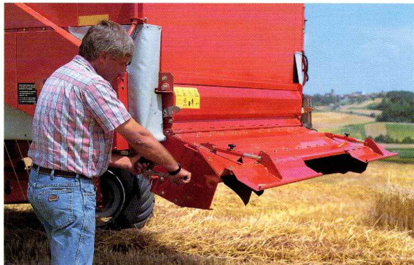
Right: The straw chopper spread pattern can be adjusted to compensate for cross-winds or hillside operation. As an option, this adjustment can be made electrically from the driver's seat
