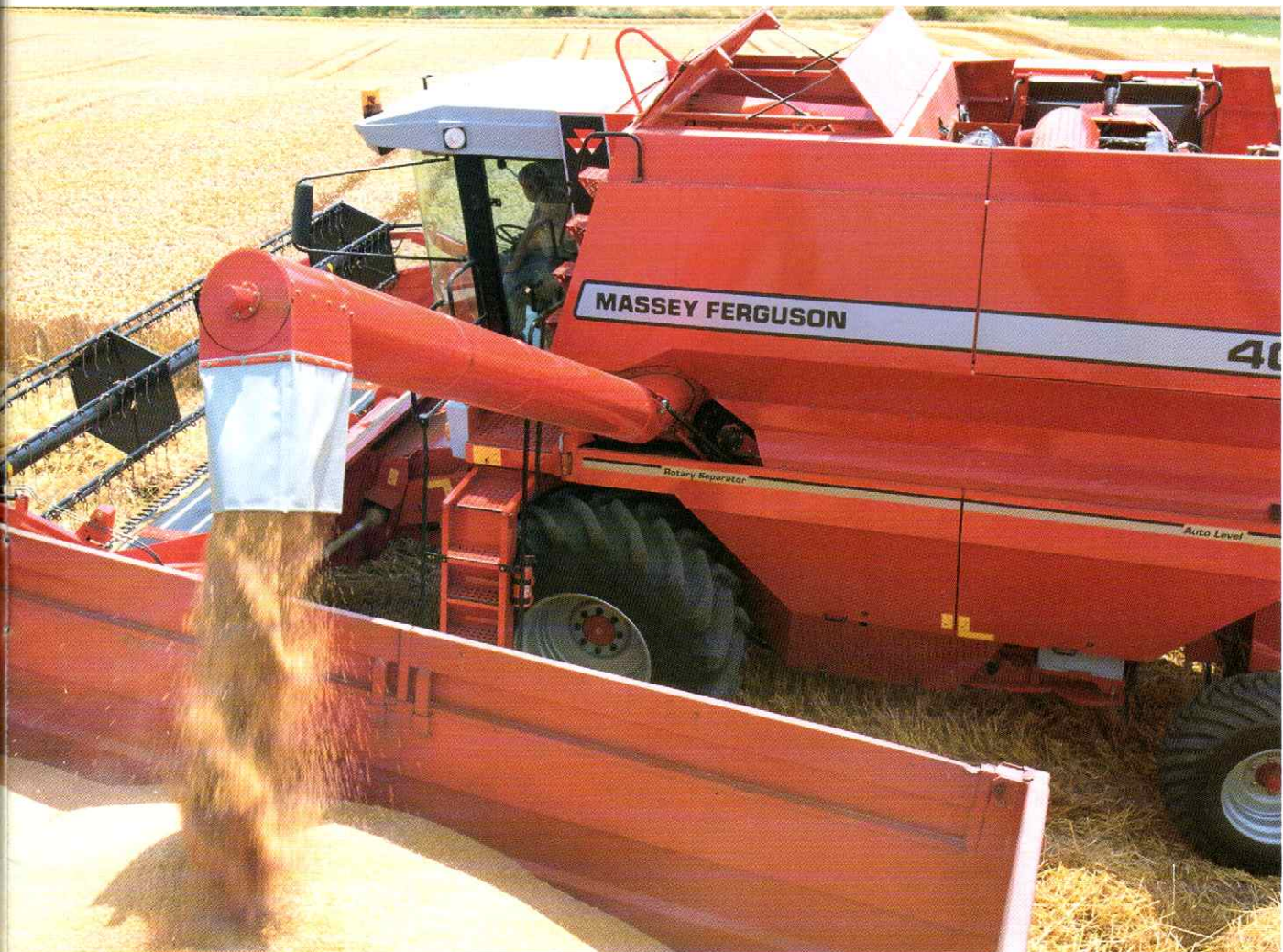
Below: Large capacity grain tanks. 7900 litre on MF 38/40. Unload a full tank in under 2 minutes
