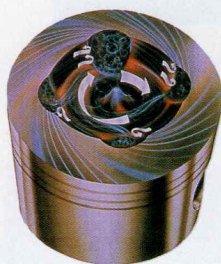
The 4-lobed piston showing the Perkins QUADRAM™ combustion design
