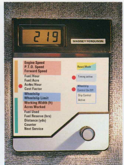
Datatronic panel, with one control for 16 functions
