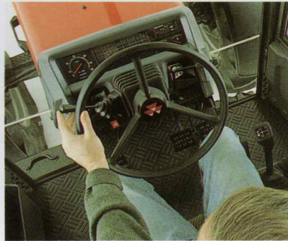
Left hand, finger-tip control of Dynashift
