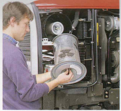
Easy access to the dual element, dry air cleaner
