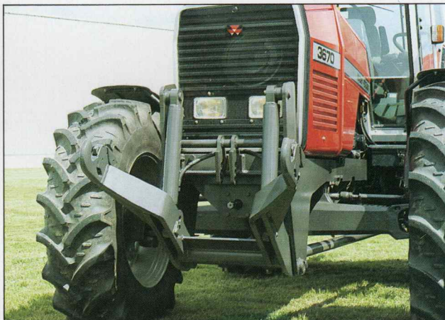
Front linkage and PTO can maximise productivity, enabling single pass, multiple operations
