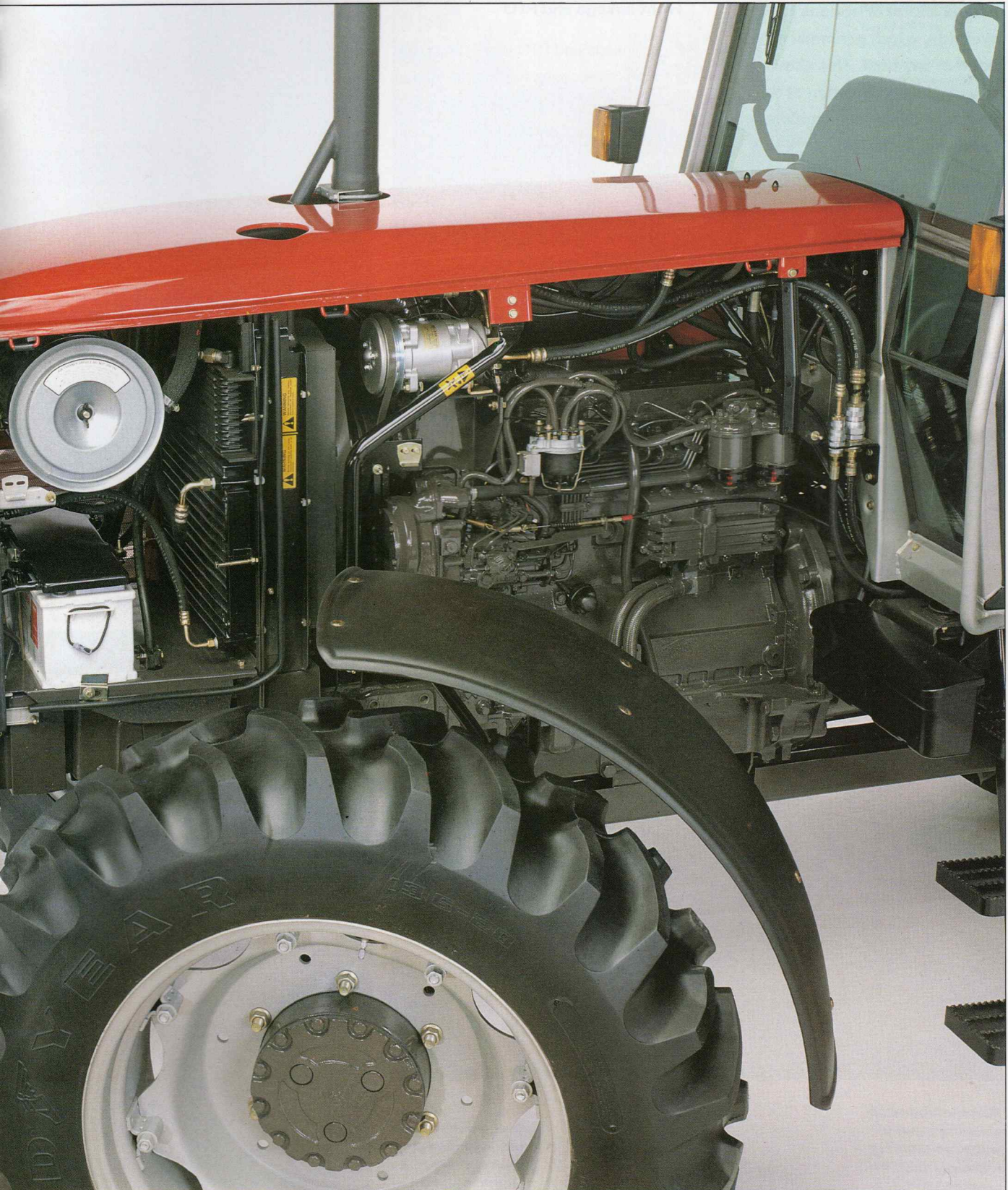
Easy access to the dual element, dry air cleaner
