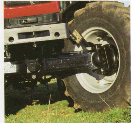
Different sizes of centre drive 4WD axle are fitted, to match tractor power (MF 8220 shown)
