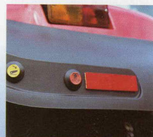
Fender mounted PTO 'Stop' control for added safety
