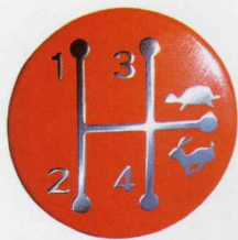
Simple gear pattern aids gear selection
