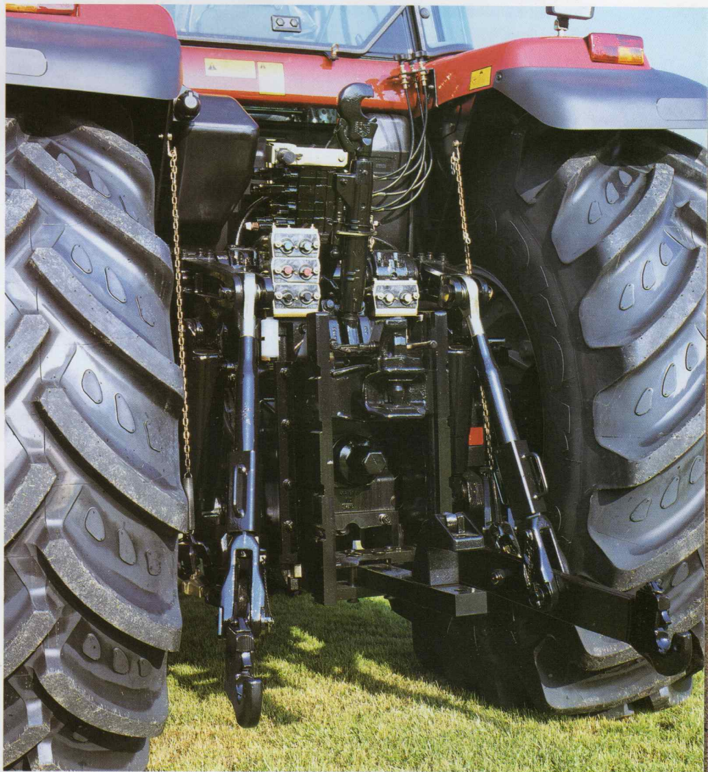
Lever-action couplers mean easy connection and disconnection, even when pressurised
