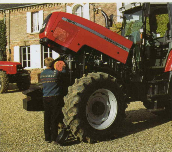
Above and right: Radiator slides clear of engine compartment for easy access for thorough cleaning. Battery and air cleaner access is good too.
