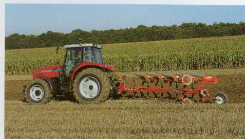
Above: ELC gives almost instantaneous response to draft signals, for precise ground contour following.
