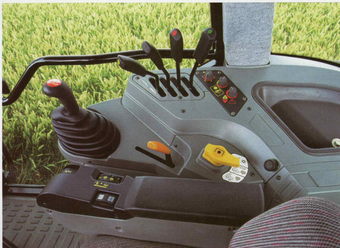
Layout includes armrest mounted controls (Dynashift model shown)
