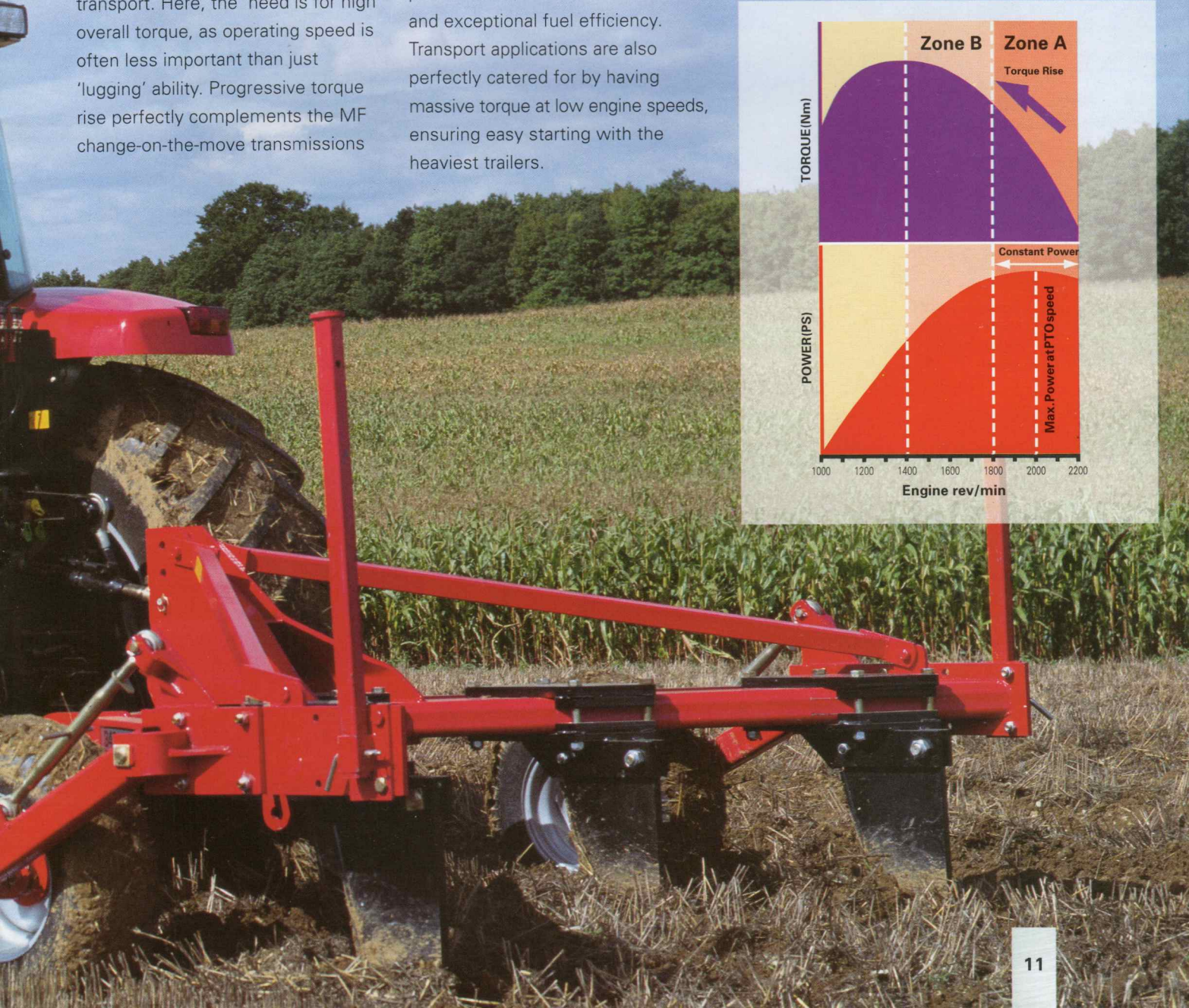
Below: The curve shows the ideal power and torque characteristics of MF's Dynatorque engines
