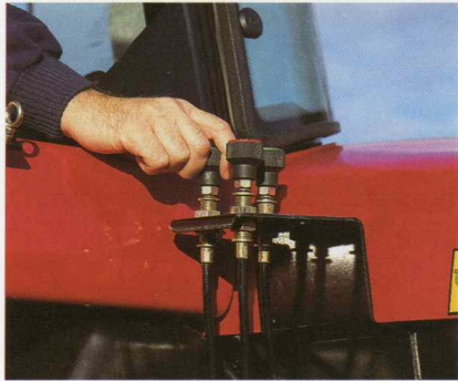
Each spool valve has individual flow control from the driver's seat
