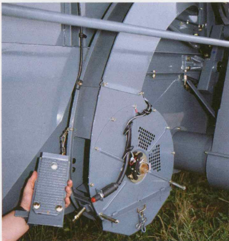
Left and right hand threshers feed returns back to the main grain pan
