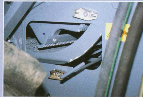
With easily removed inspection hatches, the filler plates are in with just the turn of a lever
