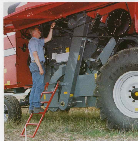
Easy opening, large side panels for easy machine settings and maintenance
