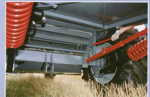
A large stone trap protects the combine from potential damage
