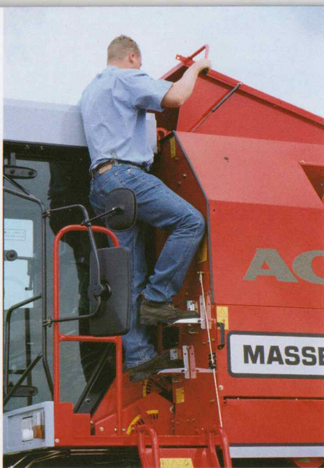
Grain tank capacity and visibility are easily increased
