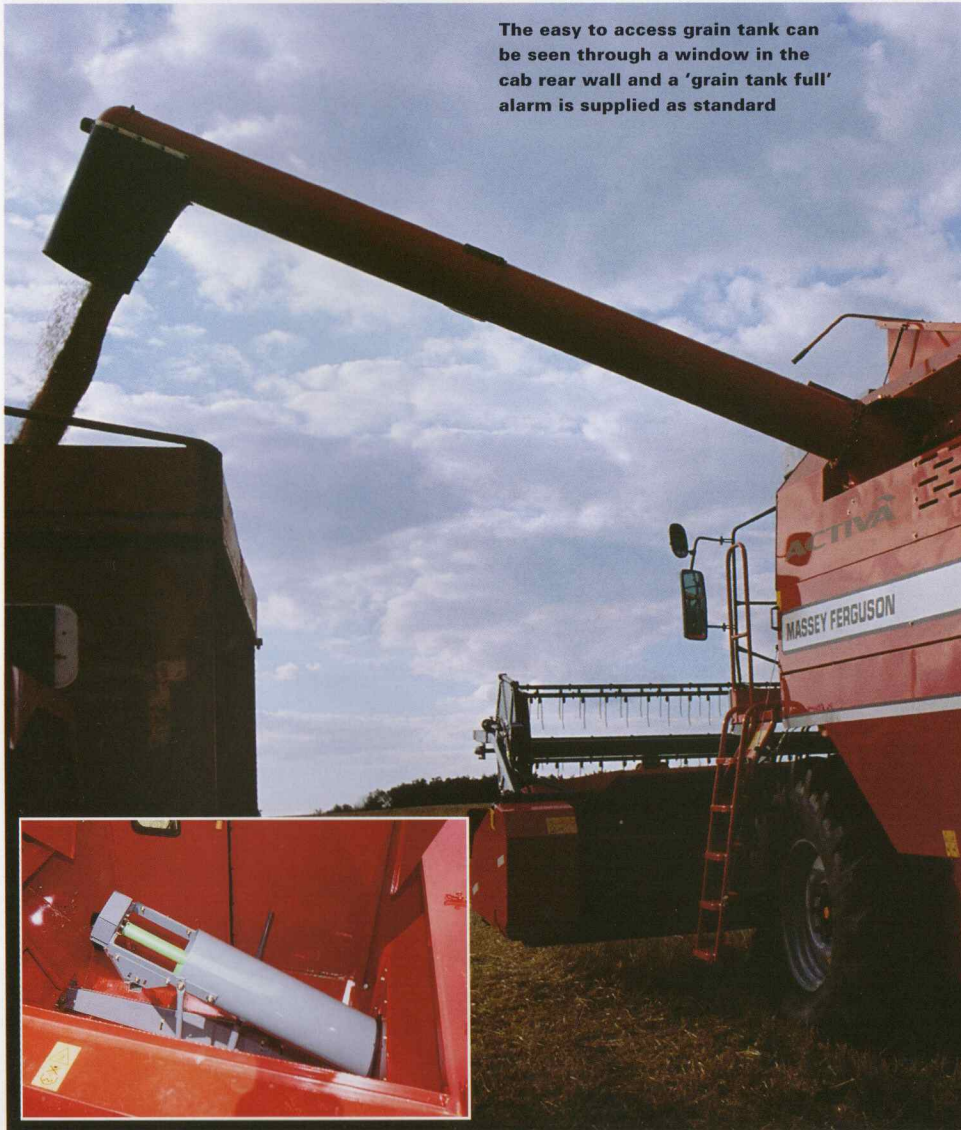
Adjustable unloading auger cover improves unloading performance
