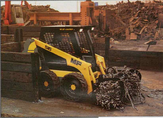
The scrap grapple allows for the safe handling of all manner of waste materials, from swarf to scrap paper.
