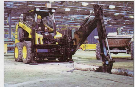
The MF516 with backhoe attachment is equipped to accurately trench in extremely confined spaces, but, unlike a mini excavator, still has the versatility to carry other attachments required on the site.
