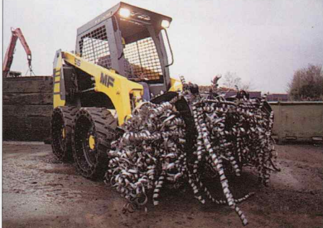
The scrap grapple allows for the safe handling of all manner of waste materials, from swarf to scrap paper.
