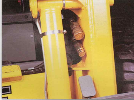
The auxiliary couplings are well protected whilst remaining easily accessible.
