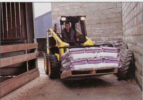
The pallet forks attachment allows palletised material to be handled in and around the farm, and enables trucks to be loaded or unloaded quickly and safely.
