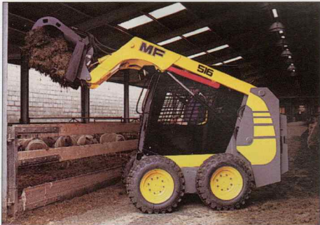
The versatile fork and grab can handle a wide range of materials, from bundles of fence posts to hay, silage, manure and hedge trimmings or loose vegetation.
