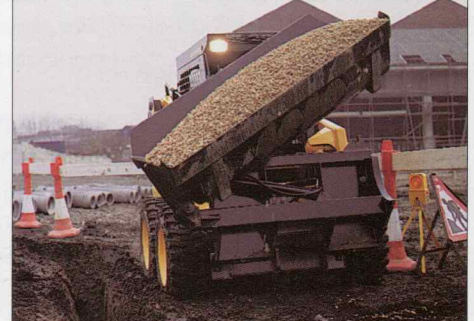
A variety of specialised buckets are available to suit specific tasks, examples include side-tip and high tip buckets, light material buckets and 4-in-1 buckets.
