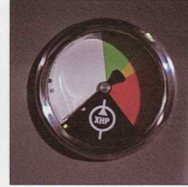
The high flow hydraulic performance gauge allows the operator to achieve optimum trenching productivity, regardless of trencher angle or ground conditions.
