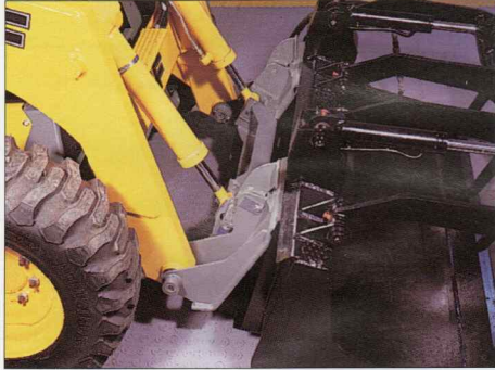
The quick attach system allows fast and safe changing of attachments.
