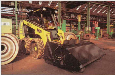
Where sites must be kept clean and free from debris, the sweeper collector attachment turns the MF516 into a highly effective tool for keeping even the most restricted areas clean.
