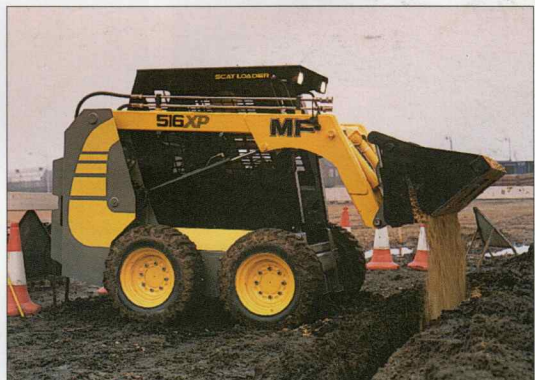
This multi-purpose bucket can perform many tasks on the work site, from backfilling trenches to landscaping.
