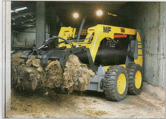
A fork and grab allows efficient handling of feedstuffs and effective general material handling.
