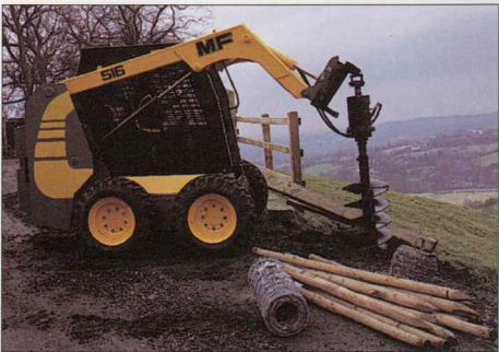
An MF516 with auger gives a compact, effective machine for fence laying operations.
