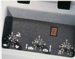
Electronic hitch controls allow fine tuning of implement operation.
