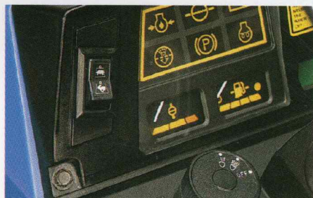
The exclusive Mode Command feature allows you to change shuttling modulation to match the job.
