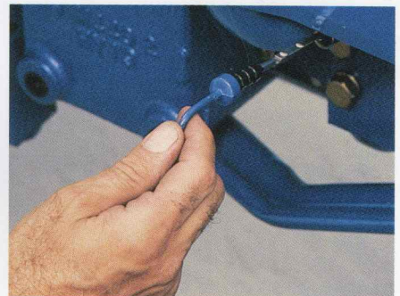
Check the oil level without raising the hood.
