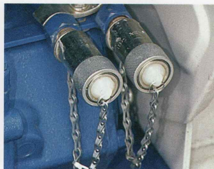
A single-spool valve lets you operate a remote cylinder or hydraulic motor.
