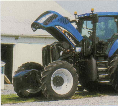
The TG flip-up hood provides ready access to the radiator, oil cooler, condenser, and air-to-air cooler.
