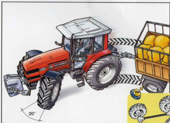
S.B.A. releases the differential locks when braking action is applied to left or right hand wheels only.
