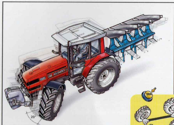
S.B.A. releases the differential locks when the steering angle widens beyond 20° at speeds below 10 km/h.
