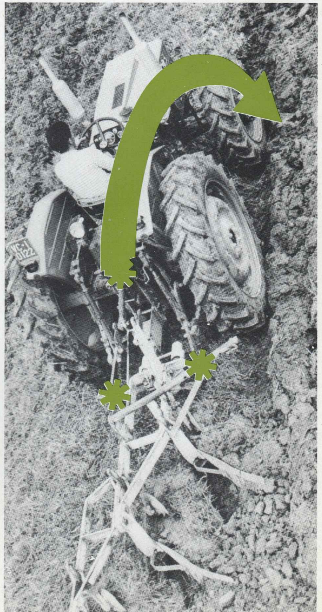
Fig. 4 - Effect of the three-point hitch on the stability of a « SAME » FWD tractor.
