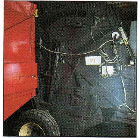
Hydraulic rams coupled to two tensioning arms
