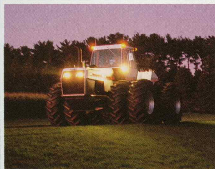
Four front and six rear lights on 4-225— eight rear lights on 4-270
