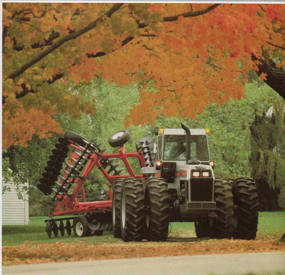
The 4-225 meets the needs of many expanding operations. It makes quick work of primary tillage chores, returns for seedbed work and stays busy right through planting, seeding and harvesting. Engine horsepower is 225, P.T.O. horsepower is 195.65.
