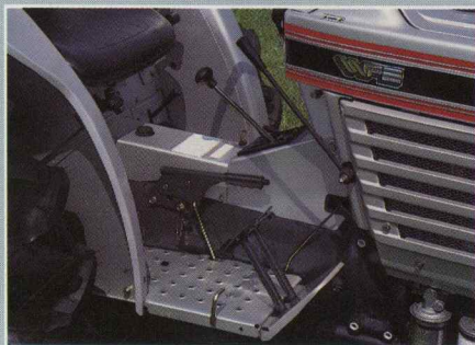
Clutch and shift with a synchronized transmission
