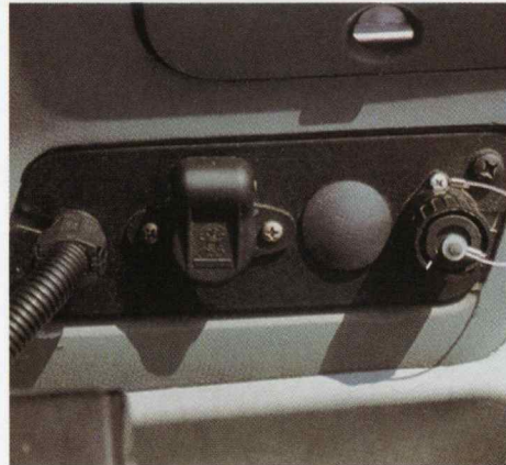
On the right of the driving position, a 25A DIN socket for electronic connection of implements is available, as well as an ISO 11786 socket for transmitting data to tractor attachments (e.g. PTO speed, forward speed etc.).
