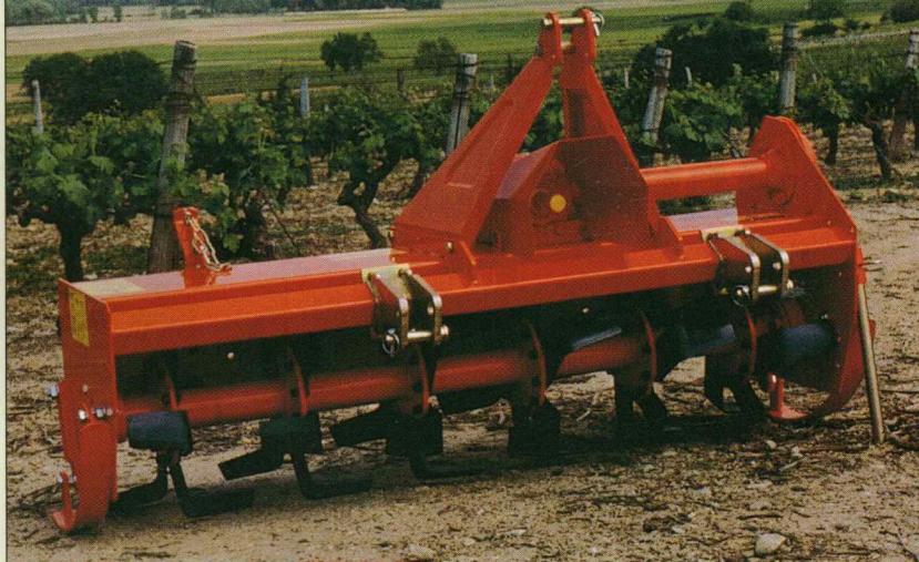
▲ HR10. Sizes: 1.06 to 1.8m. For tractors 17kW (23hp) to 35kW (47hp).
