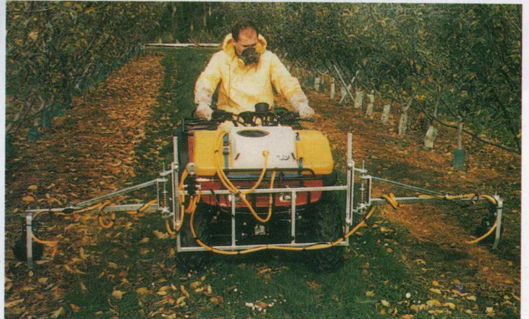
BSLV. Low volume, inexpensive band spraying with all the attributes of CDA. Coverage: From 1.0m.
