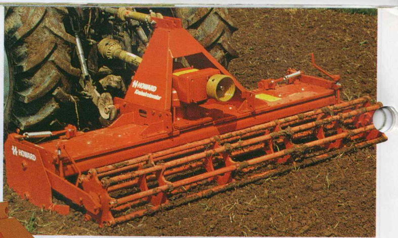
▲ HK20. Sizes 1.55 to 3.0m. For tractors up to 70kW (95hp).
