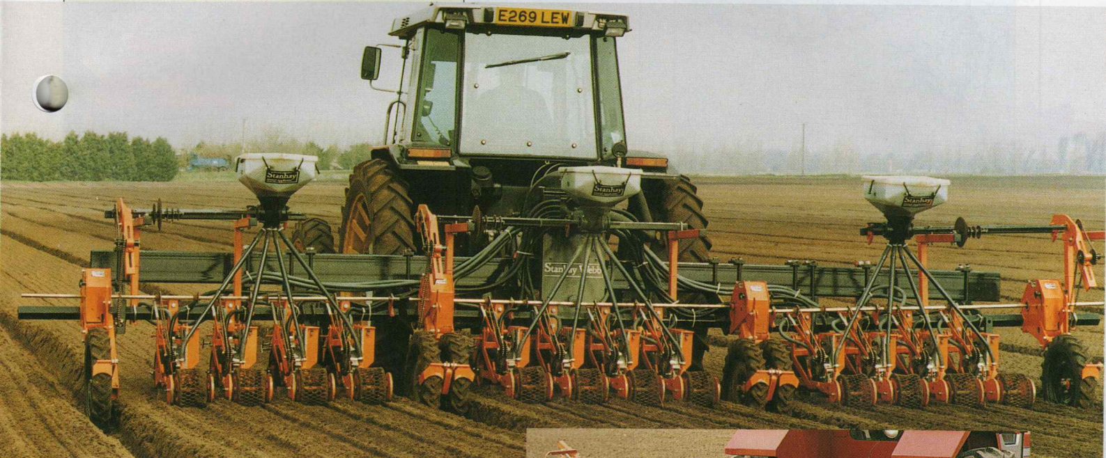
▲ SINGULAIRE 785 ROW UNIT Clod deflector and cage rear wheel are optional. Single or multi-line coulters available.
