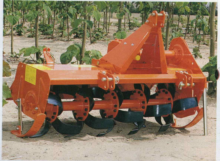
HR8. Sizes 80cms to 1.25m. For tractors up to 33kW (45hp).
