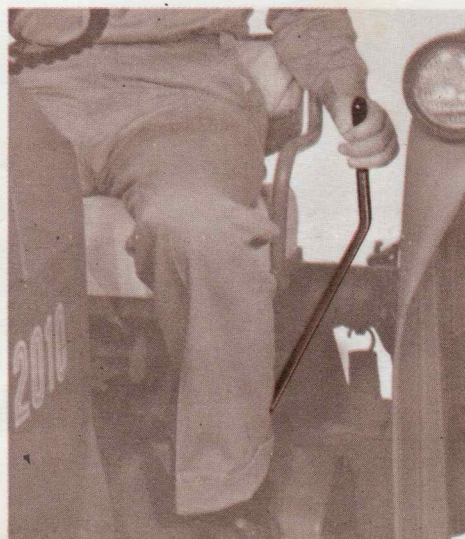
Below: You can stop or start the power takeoff on the "2010" instantly with this handy clutch lever.
