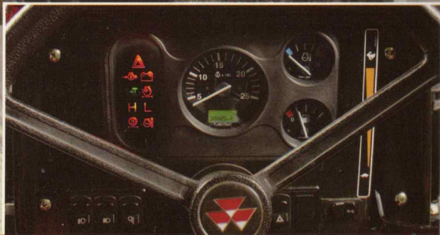
The instrument panel's logical layout, with digital hour meter and indicator light cluster, provides at-a-glance access to important operating information.
