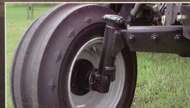
Front axle spindles are nearly 4" shorter on 2WD models, lowering the center of gravity, increasing maneuverability and traction, and providing a lower overall height.
