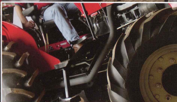
The exhaust system incorporates a horizontal design that runs below the operator's platform and exits near the rear axle. This low-profile feature also provides unobstructed views, for improved visibility.
