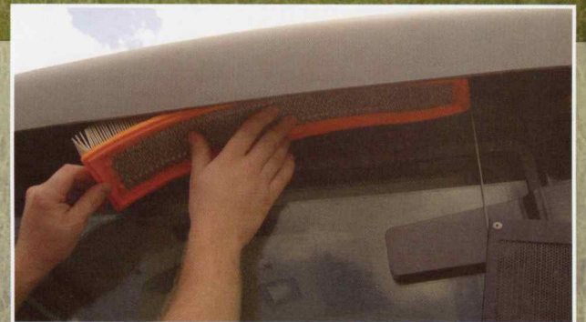
The cab air filter, located just above the entrance door, is easily serviced and maintained.
