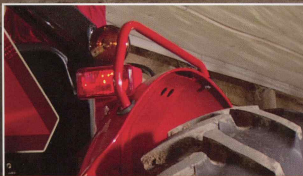
Rear lighting, mounted on the dished rear fenders, is protected from low branches or obstacles by a fender-mounted guard rail. The narrower fenders reduce height over the rear tires and create a slim profile.
