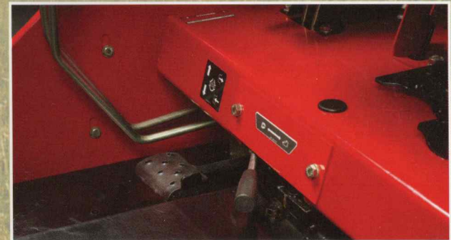
Combining Valve – Combines the flow of the Ferguson 3-point pump and the auxiliary hydraulic pump. Optional on the 533, 543 and 563.
