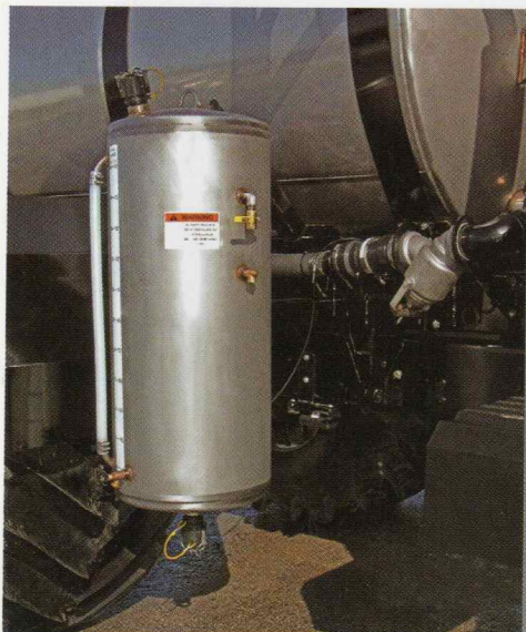
Easy access to primary strainer and flow meter
