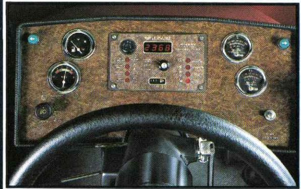
Narrow designed instrument panel for high knee clearance. Conventional gauge and warning lamp system provides you with accurate, on-the-go information and warns you of potential trouble. Rotary knob on the panel allows you to select engine, ground and PTO speed.
