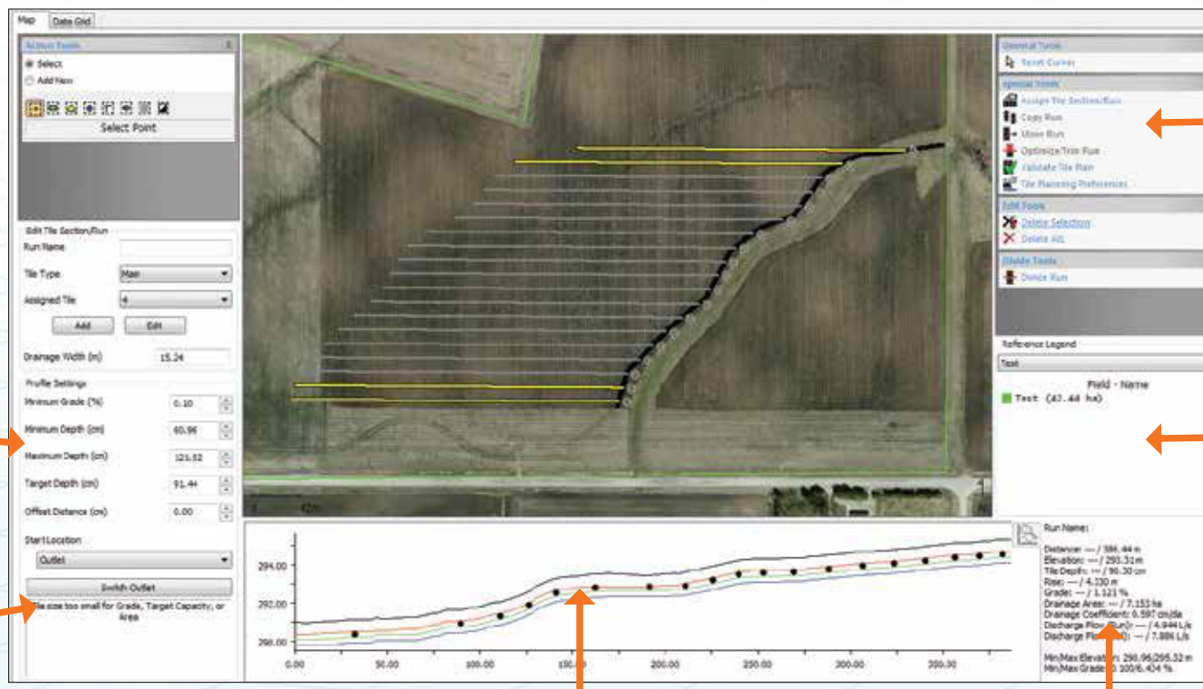
Soil profile showing soil surface, placement of the tile run and connections.
