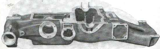
One piece main frame of Case 10-18 Tractor
