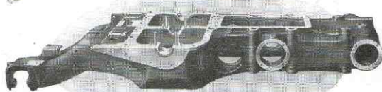
The one piece main frame of the Case 15-27 Tractor
