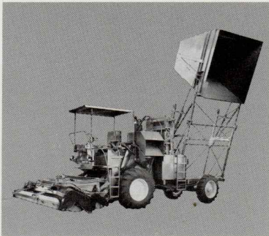
Bulk Product Hopper fully extended for emptying
