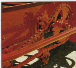
Strong extended pitch chain drive
