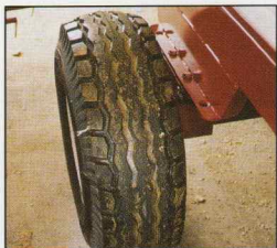
Lugged flotation tyre and adjustable axle
