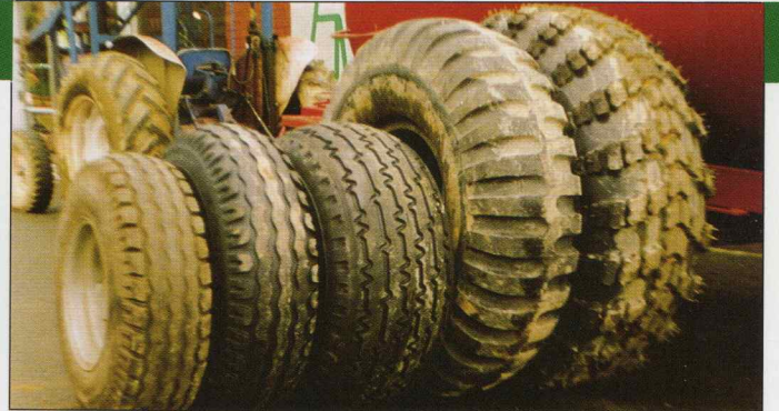
Tyre sizes left to right: 10/75 x 15.3, 11.5/80 x 15.3, 400 x 15.5, 1400 x 20, 1300 x 530
