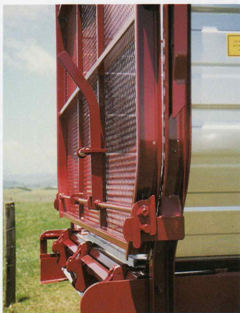
Self-releasing back gate for rear unloading.
