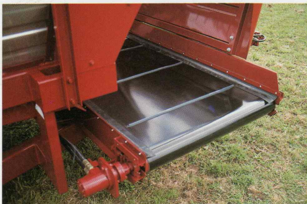
Adjustable cross conveyor bed with priority oil flow.
