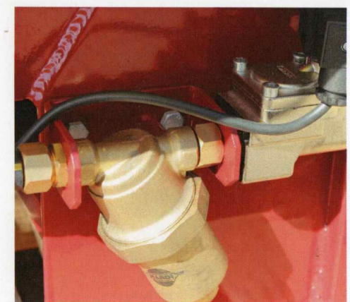
Pressure filter: Prevents residue from blocking nozzles. Easy access for cleaning - fitted standard on the ZEBRA.
