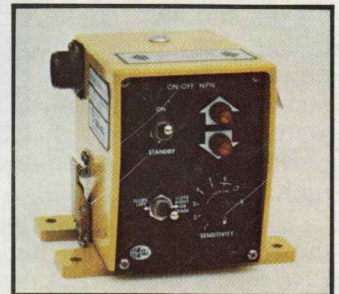
The microprocessor control for the Twin Disc transmission was manufactured by Grad-Line, Inc. The controller senses the position of the shift lever, clutch pedal and determines the proper range.
