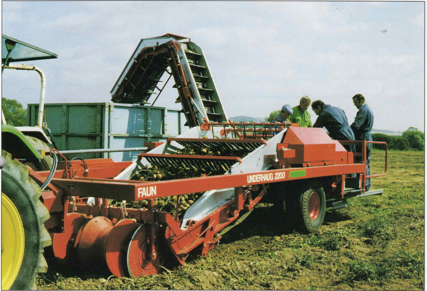
Kverneland Faun 2220 two row potato harvester in operation. Illustrated with an inspection/sorting table for up to 4 operators.
